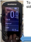
To switch on/off the light on your e-bike, press and hold the button on the right side of the display until the light goes on/off.
