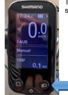
To switch on/off the light on your E-Bike, press and hold the button on the right side of the display until the light goes on/off.
